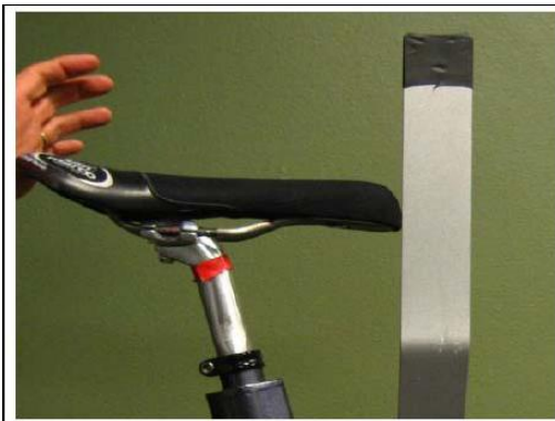
This saddle meets the standard dimension limits. It is 5 cm behind the bottom bracket axle.
