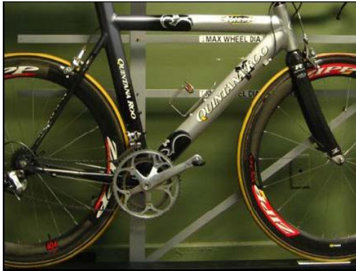
The Bicycle above is legal. It has a double triangle configuration.
