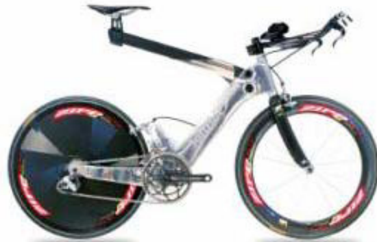
The Bicycle above is not legal. It has no seat tube or seat stays.
