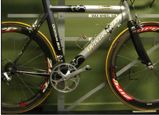
The Bicycle above is legal. It has a double triangle configuration.
